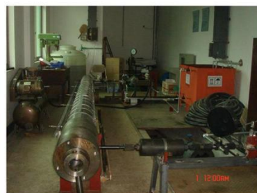
Super-high pressure testing autoclave for CSIC 715 Ø130×5000mm; 200MPa; 250℃
